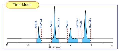
In time mode, the valve is operated according to a preset time program. The valve is switched repeatedly, and the eluent in arbitrary times ( ) is sent to waste.
