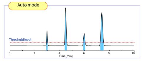
In auto mode, peaks were automatically detected by setting a threshold level. Only when the signal from the detector exceeds the threshold (Blue area ()), the eluent is sent to waste line.
